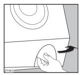
When no more water comes out, unscrew the filter and remove it.
